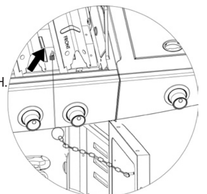
Main Burner Lighting Rod Placement
