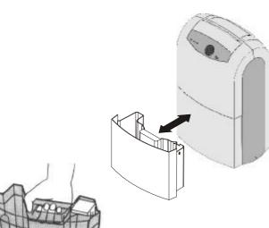
Remove the water tank, empty water, place tank back in unit and unit will return to operation mode.
