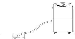
When using the continuous drain feature, make sure the drain tube is laid flat horizontally and fastened in place; avoid overlapping or depressing, and make sure it lays lower than the drain hole.
