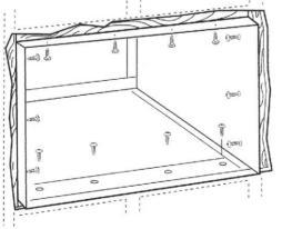
C Place the case in the wall opening and place wood support strips between the case bottom and the flashing on both sides of the bottom rail. They should be the same height as the bottom rail and the same length as the wall opening.
