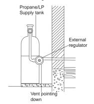
Fig.6 External Regulator With Vent Pointing Down
