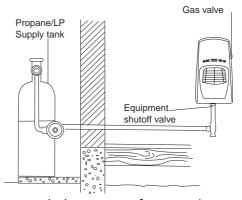
Fig. 10 Checking Gas Joints for Propane/LP Gas
