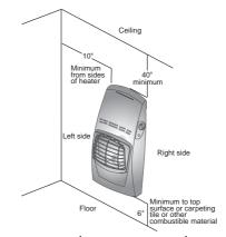
Fig.4 Mounting Clearances As Viewed From Front of Heater
