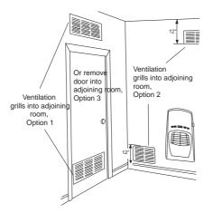
Fig.2 Ventilation Air from Inside Building
