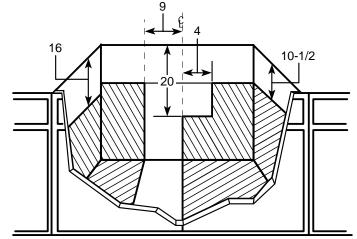
**Receptacle Location:** Install an approved junction box within shaded area shown in diagram. Junction box must be at least 10-1/2" below top of cabinet.
