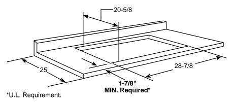
Note: A 6" minimum spacing to adjacent side wall is required
