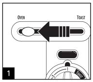
Make sure Mode Selector is in "OVEN" position (slot closed).
