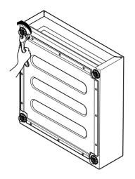
**9** Remove four (4) screws (two on each side) on both side of slide.
