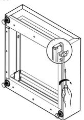
Remove twelve (12) screws on the bottom of the pedestal.
