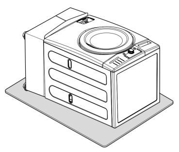
2 Open the drawer, and then remove the four (4) screws (two on each side) on both side of drawer.
