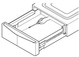
Remove two (2) screws on the either side of the drawer.
