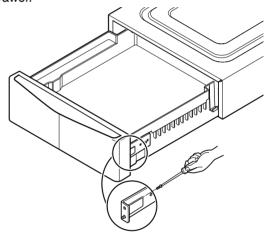
6 Remove six (6) screws on the front cover assembly.
