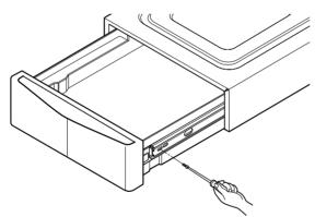
**Q** Pull up the drawer to disassemble.
