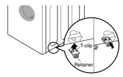
Position dryer on top of the pedestal.
