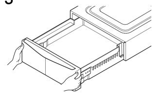
A Remove three (3) screws on the drawer.
