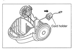
2) Lift the cord reel assembly from the body base in the direction of the arrow.
