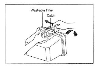
Pull the mesh screen down from the washable filter.
