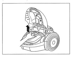
2) Hold the handle of the washable filter and pull it out of the dust bin.
