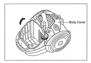
3) Strip off the lead wires from the motor & cord reel.
