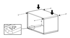
• Insert the rear grille and fasten the 8 washer screws as shown below.
