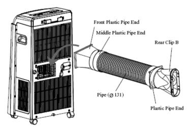
The exhaust hose should be kept as short and straight as possible. Prevent any sharp bends in the exhaust hose, as this will trap hot exhaust air and cause the unit to run less efficiently.
