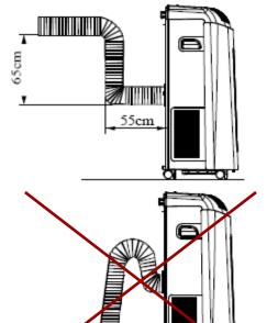
The hot exhaust air can be vented through the wall or out a window. If mounting in the wall, the height of the hole should be 16 to 50 inches (40cm to 130cm).
