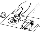
You may check to see if you need to add rinse agent by removing the fill cap and looking into the container. You may also check the rinse agent, on some models, by pressing the clear center of the fill cap 2 or 3 times. If rinse agent is drawn into the center of the fill cap, you have enough. If the center area remains clear add rinse agent. Your dishwasher's rinse agent container holds approximately  $4\frac{1}{2}$  ounces. This should last about 3 months. Fill as needed.
