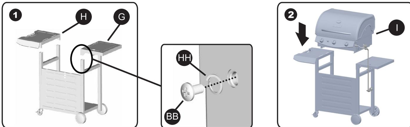
3) Install the grill housing assembly using **six** washers (GG), lock washers (HH), and M6x12mm screws (BB) as shown. First insert the back screws in an alternating pattern (install one screw on the left then install the next screw on the right side).
