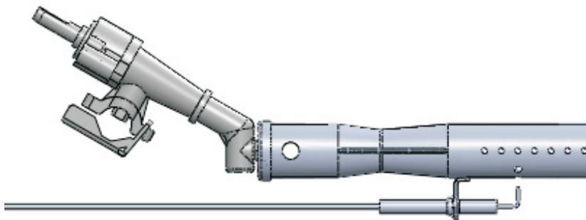
1. Overlap 20mm between venturi tube and nozzle when assembled.
