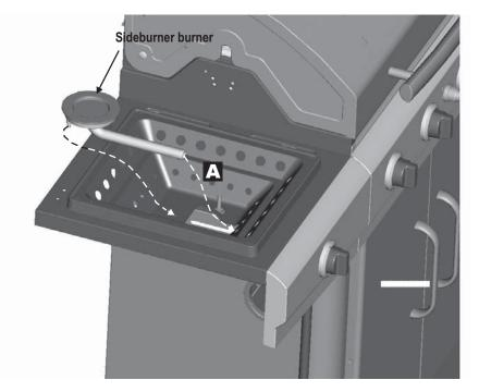
Attach and fully secure hinges to lid with four #8-32x3/8" screws, #8-32 flange nut first. Place sideburner lid onto left side shelf and align hinges to holes on side shelf top. Attach sideburner lid assembly to side shelf using four #8-32x3/8" screws, #8-32 flange nuts.
