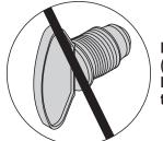
Do not use a POL transport plug (plastic part with external threads)! It will defeat the safety feature of the valve.
