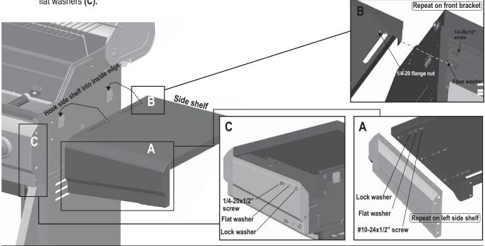
Repeat step 7(A) on left side shelf. Hang sideburner shelf on the tabs mounted on the firebox. Attach shelf brackets to cart side panel using two1/4-20x1/2"screws, fiber washers and 1/4-20 flange nuts on each bracket (A). Secure fascia to firebox using two 1/4-20x1/2" screws, 7mm lock washers and 7mm flat washers.
