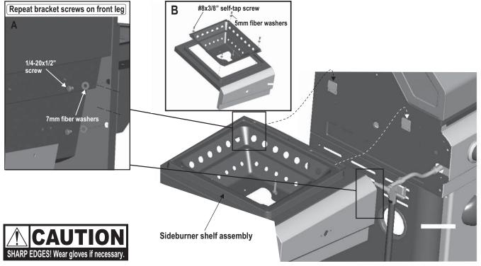
First, remove the two screws from the sideburner valve bracket. Align sideburner valve bracket behind sideburner shelf fascia with bezel on same level. Secure them altogether with two #8-32x3/8" screws. Press sideburner control knob onto valve stem.
