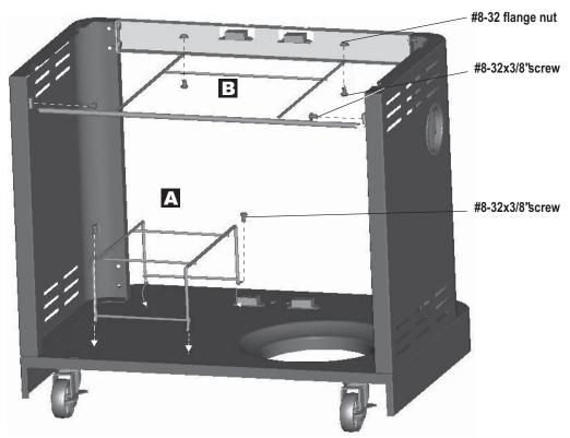
First two #8-32x3/8" machine screws are installed partially in the cart side panel (A). Slide the door hinges onto the screw with arrow direction as indicate. Secure the right door with four #8-32x3/8" machine screws. Repeat same steps on the left door. Slide the condiment baskets into brackets at back of doors.(B)
