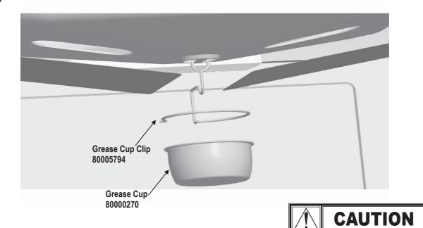
Failure to install grease clip and cup will cause hot grease to drip from bottom of grill with risk of fire or property damage.
