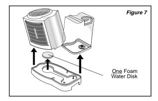
7. Rinse Base thoroughly. Place *Only One* New Foam Water Disk into Base Well. Reattach the Humidifier Body Assembly and Water Tank to the Base.
