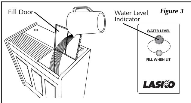
**When filling the Humidifier for the first time:** Fill with 5 gallons of cool tap water. (The Humidifier's Water Tray only holds 5 gallons at one time. DO NOT PUT IN MORE THAN 5 GALLONS OF WATER!)
