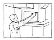
3. Drill the four (4) mounting hole locations. They are marked with a +. Cut the inside opening of the mounting template, leaving the outside lines visible. Be careful to avoid injury from sharp edges. See sketch #726
