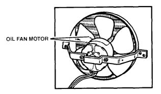
**4.** Oil the motor through the tubes provided. An easy to use capsule of especially recommended oil (Part Number 10943) is available through your nearest Whirlpool Factory Service Center, or use SAE #20 non-detergent oil.
