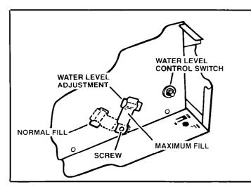
The Water Level Control Switch will automatically turn off the dehumidifier at the fill level you selected when pan is properly placed. Loosen the screw to move the Water Level Adjustment. Retighten screw when adjusted.
