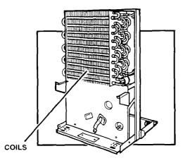
2. Coils should be inspected annually. Brush clean, if necessary, with warm water and mild detergent. Rinse and dry. **Be sure power supply cord is disconnected.**
