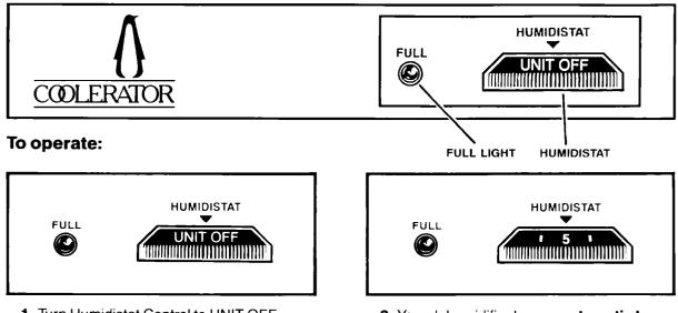
2. Your dehumidifier has an **automatic humidistat.** Turn Humidistat Control left toward DRYEST for normal operation. Set at number 5 or 6 to start. Adjust later, if necessary.
