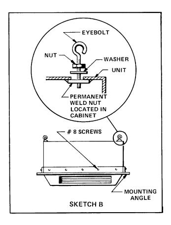
6. Lift unit into place and support unit while securing to permanent ceiling, ceiling joists, etc. See Sketch C.
