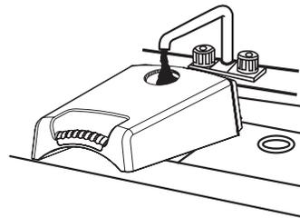
4. Listen for air bubbles. Look for leaks around the "Side Fill Cap" and valve plunger.
