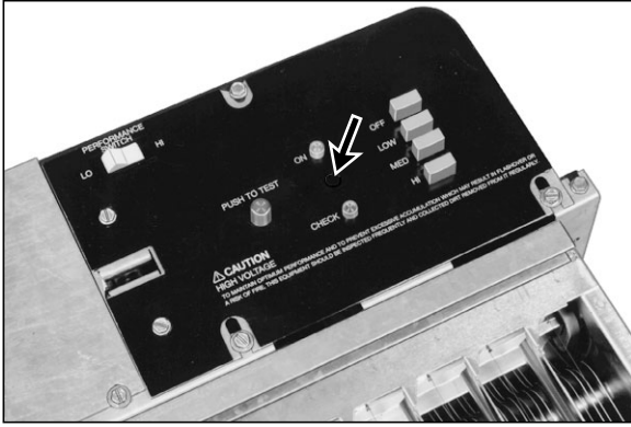
1. LOCATE WASH LED CUTOUT BEHIND SWITCH COVER ASSEMBLY STICKER.
