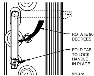
**Fig. 16. Install handle on end of cell closest to access door.**
