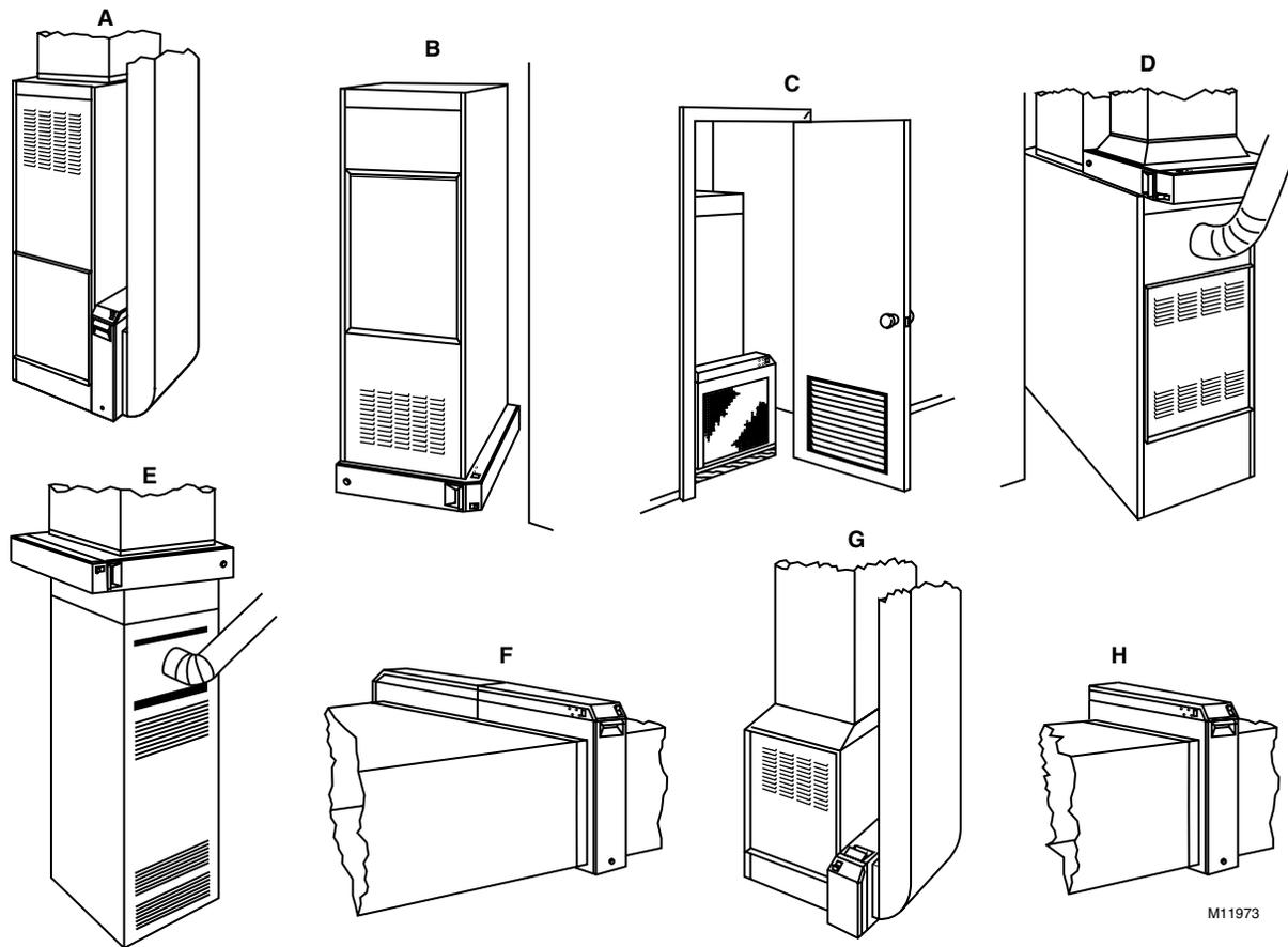
Fig. 3. Mounting positions with variety of furnace installations.
