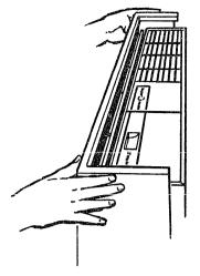
3. Lift the room cabinet, position the top of it onto the front lip of the top air discharge grille, and press it down to secure it.
