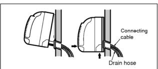
Press the lower left and right side of the unit against the Installation Plate until the hooks engages with their slots (sound click).
