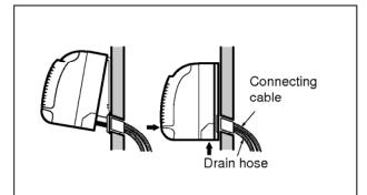
Press the lower left and right side of the unit against the Installation Plate until the hooks engages with their slots (sound click).
