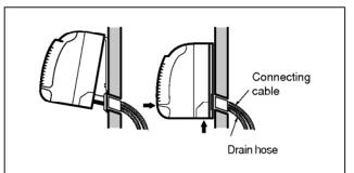
Press the lower left and right side of the unit against the Installation Plate until the hooks engages with their slots (sound click).
