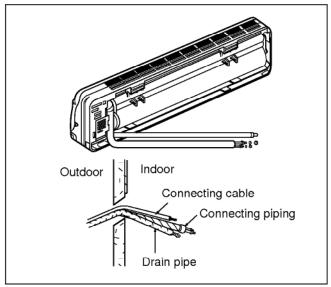
6. Tape the tubing, drain hose and the connecting cable.
