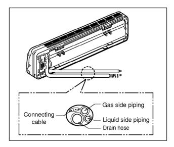
Tape the tubing, drain hose and the connecting cable. Be sure that drain hose locates at the lowest side of the bundle.
