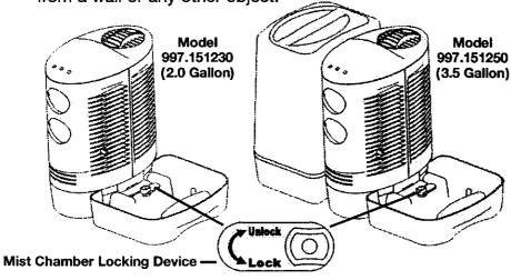
Remove the tank(s) from the base by grasping top handle. Rotate the mist chamber locking device to unlock the mist chamber (see illustration above). Lift the mist chamber off the base. Locate the absorption sleeve attached to the heating element on the underside of mist chamber. Be sure the sleeve is tightly attached to the heating element. Loosely attached absorption sleeves may produce less humidity and cause malfunctions.
