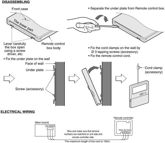
The maximum length of the cord is 100m. If the length of the cord exceeds 50m, use a wire size greater than 0.5mm<sup>2</sup>.
