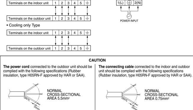
If the supply cord is damaged, it must be replaced by a special cord or assembly available from the manufacturer of its service agent.
