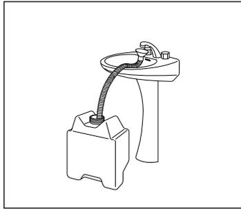
B) Turn the tank upside down and remove the plug. Remove the extendable tube and fill the tank, leaving it on the ground.
