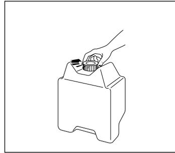
C) After completing the filling procedure, replace the extendable hose and the cap and screw it in tightly. Return the tank to its place, with the writing FRONT clearly visible. Carefully hold the panel in the center and lower to its closed position.
