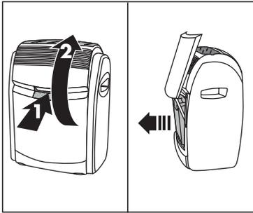
A) To open the front panel **3** grip the side panel and gently pull the panel towards you and upwards. Remove the tank **5**. Lift it forward.
