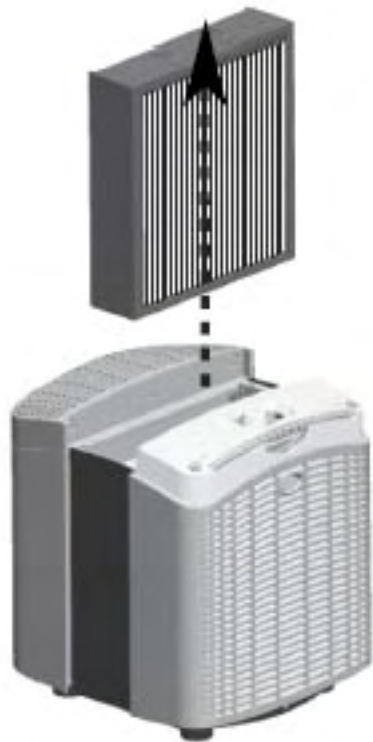
Fig. 7 - Removing the Main Filter
