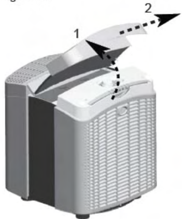
Fig. 4b - Removing the Top Cover
