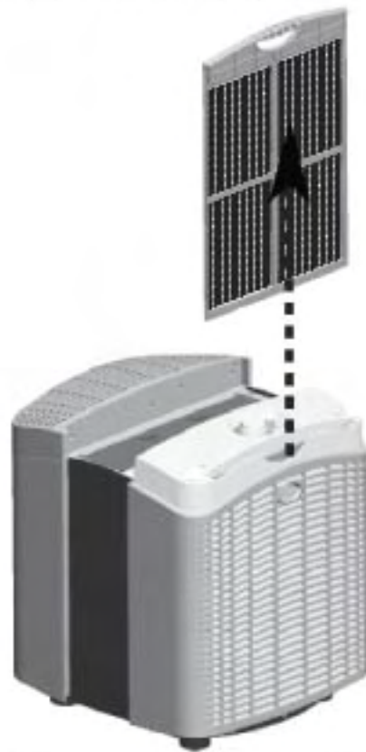
Fig. 5 - Removing the Pre-Filter
