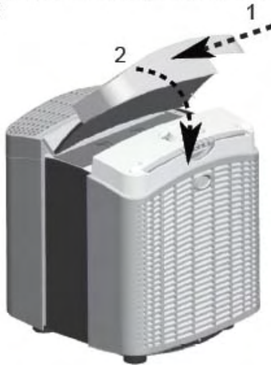
Fig. 10 - Reinstalling the Top Cover
