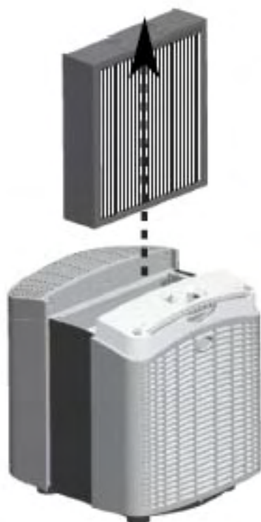
Fig. 7 - Removing the Main Filter
