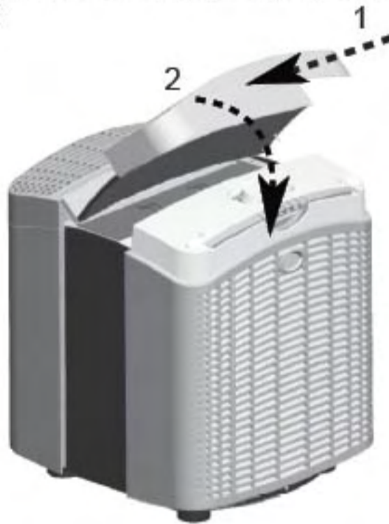
Fig. 10 - Reinstalling the Top Cover
