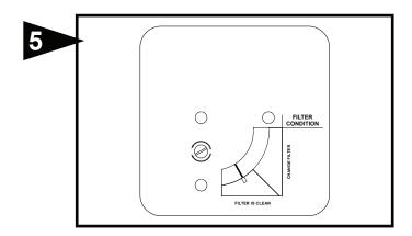
Turn on electricity and run furnace blower on highest speed. Calibrate condition indicator, with a small screwdriver adjust the calibration screw to put the pointer in the center of the "FILTER IS CLEAN" range.
