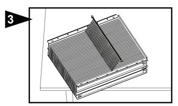
Install the plastic pleat spacers, being careful to insert one support finger between each pleat. Press each end of the pleat spacers down firmly to fully engage the media frame. Pleat spacers may snag on air cleaner cabinet if not pressed down below media frame rail.
