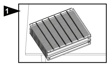
Turn off electricity to furnace. Pull front cover off and slide media carrier out of air cleaner cabinet. Place air cleaner media frame on table with plastic pleat spacers on top. Loosen pleat spacers by gently lifting at each end. Carefully remove all pleat spacers. Lift used air cleaner media out of frame for disposal and clean media frame.
