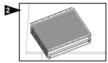
Place new media pack (Part No. 13156) onto the media frame. Slide media pack toward foam gasket. Line up holes in the cardboard strips with the holes in the media frame.
