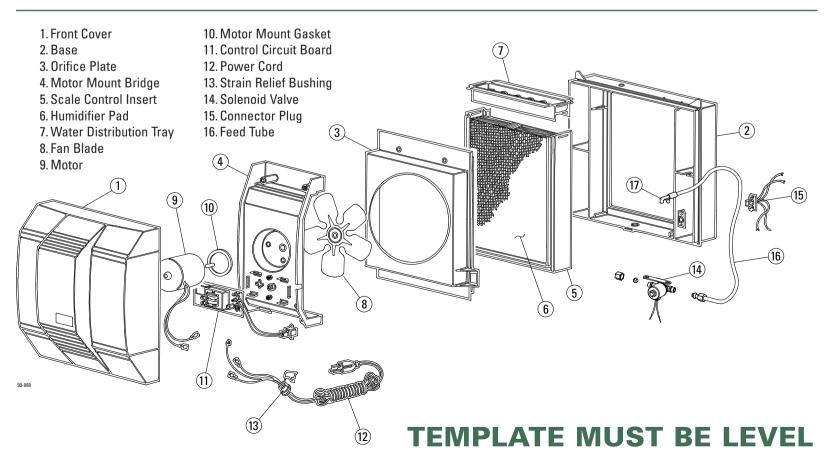
**7.** The humidifier power cord must be plugged into a 120 VAC outlet. Wire an electric outlet box to power source other than furnace fan motor circuit. Outlet box can be powered off of the 120 VAC line **before** it enters furnace.
