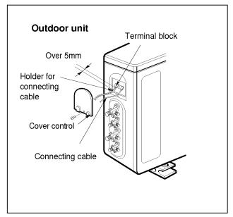
The power cord connected to the outdoor unit should be complied with the following specifications (Rubber insulation, type H05RN-F approved by TUV or VDE)
