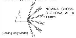
The connecting cable, from the indoor unit to the outdoor unit should be complied with the following specification.(Rubber insulation, type H05RN-F approved by TUV or VDE)
