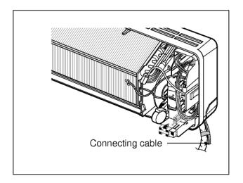
The connecting cable, from the indoor unit to the outdoor unit should be complied with the following specification.(Rubber insulation, type H05RN-F approved by TUV or VDE)
