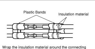
Wrap the insulation material around the connecting portion.
