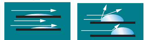
LG PLASMA Film of water allows for efficient and low noise air flow
