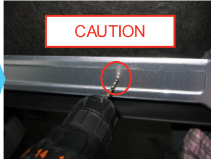
Drill the pilot hole. Be careful not to damage the door liner when drilling the hole.
