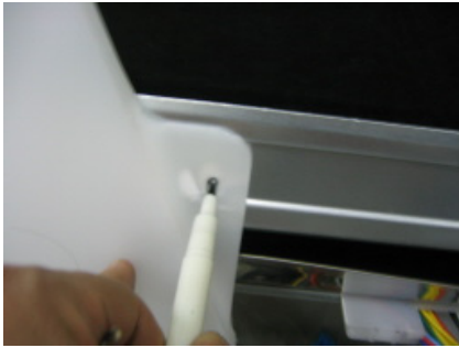
Mark the location to drill the hole. Make sure the bottom of the vent will align with the bottom of the front door panel.
