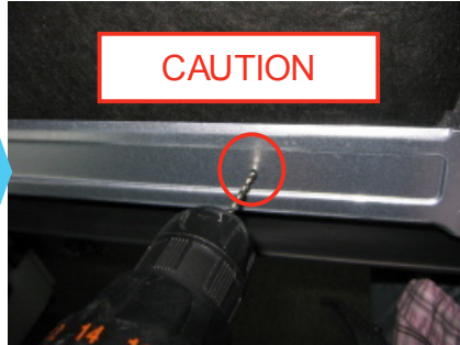
Drill the pilot hole. Be careful not to damage the door liner when drilling the hole.
