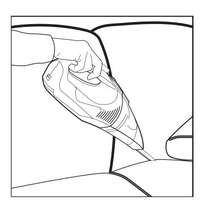
The crevice tool is stored in the base behind the hand vac (see fig. 1). Pull crevice tool away from the base and put the wide end into the end of the hand vac nozzle. (See above) The crevice tool is used to clean corners, baseboards, between cushions.
