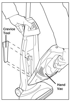
1. To remove the hand vac from the base, push in on the hand vac release button, and tilt hand vac out of base as shown above.
