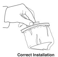
NOTE: If filter is not properly installed, dirt and dust will go past the filter and this can damage the cleaner motor.
