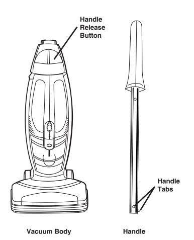
1. Remove vacuum body and handle from carton. Locate the handle release button on body and the handle tabs on handle.
