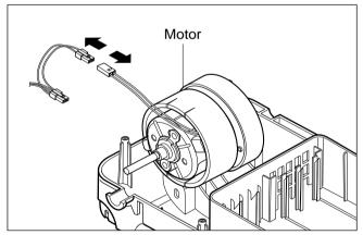
Disconnect wires and disassemble switch, fuse and power cord.
