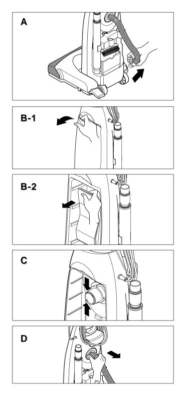
Open dust cover and remove filter bag.
