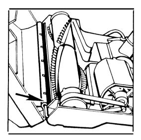
While maintaining front connection, rotate cover over nozzle base and pull nozzle cord through opening in cover.
