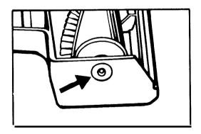
Position round projection on end of agitator (opposite the belt) into the opening on the wall of the nozzle base. Slide belt side of agitator into place, pushing the agitator slightly to left, pulling it forward and then down.
