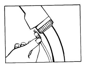
Connect nozzle power cord to receptacle underneath handle.
