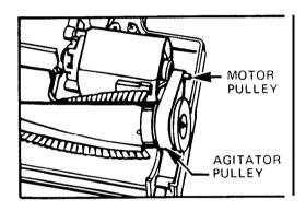
Place one end of new belt around the motor pulley, with lettering on outside of belt.
