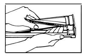
To remove the agitator, position your hand underneath the nozzle base at the agitator opening and push up the belt side of the agitator. Remove agitator and old belt.
