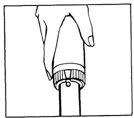
To attach the hose to the extension wands, rotate the plastic latch ring on the handle to accept the button projection on the curved wand.
