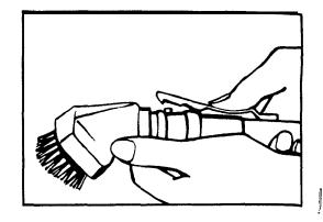
Tools may also be attached to the handle by rotating the plastic latch ring to accept the button projection on the tool. Then, turn the latch ring as shown to lock the tool in place.
