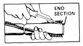
2. Pull or pry out end sections as shown in illustration.
