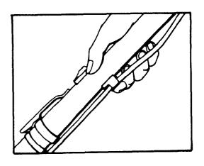
Attach the curved wand to the straight wand. Position cord into cord clips on extension wands, placing excess cord between nozzle and bottom cord clip.
