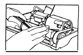
The cover attaches at the front of the nozzle. Place the notched edge at the front of the cover into the groove in the nozzle base.
