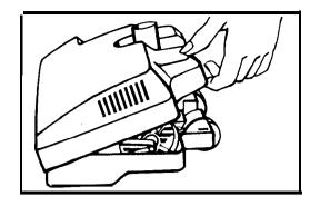
Return nozzle to original position and lift up back of nozzle cover. Then remove cover, rotating it forward and lifting it off.
