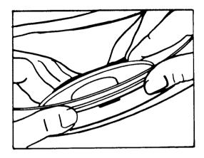
Grasp edges of collar section and push opening of collar section of new bag onto holder. Make sure collar is pushed completely up to the ridge on the holder.
