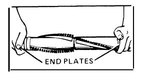
1. Hold agitator as shown. Turn end plates counterclockwise until one end plate comes off.
