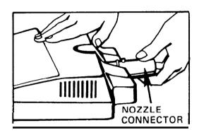
Disconnect cleaner from electrical outlet and disconnect power nozzle from extension wands.
