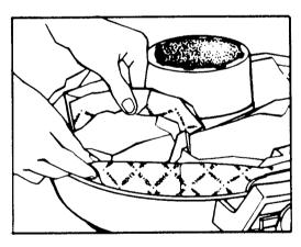
Adjust bag around the motor housing and open the folds of the bag to allow the bag to properly fill. Make sure all four folds are open.
