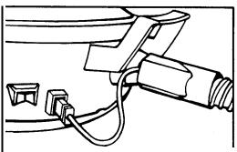
To disconnect hose, first remove hose cord plug from receptacle. Then, depress latch away from hose connection opening in cleaner. While holding latch, turn the hose counterclockwise until the arrow lines up with dot on the cleaner.
