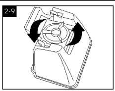
Carry tank to a sink. Rotate tank cap counterclockwise and lift up to remove cap.
