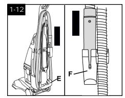
Continue wrapping hose under lower hook (E). Snap hose end **fully** into holder (F).
