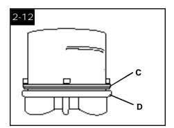
If rubber ring (C) on cap has become dislodged, reposition it with uneven side against ledge (D) as shown.
