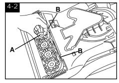
Grasp inner portion of brush (A) and pull brush assembly out slightly to reveal latches (B).
