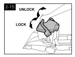
Raise handle to carrying position (straight up) to **unlock tank** from base of deep cleaner. Lift tank from deep cleaner and carry it to a sink or drain.
