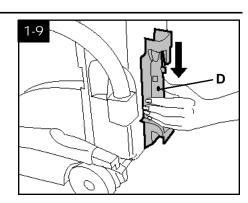
Slide rack down into place. Insert screw at (D) and tighten with a Phillips screwdriver.
