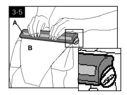
2. With foam strip (A) (located under the netting) in position as shown, place attachment on front of nozzle (B). Make sure arrow on end of attachment points in the direction as shown.
