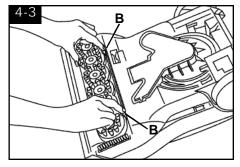
Press both latches (B) and pull brush block out. The brushes can be cleaned under running water.
