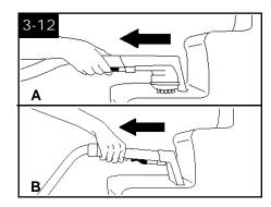
9. Lift tool, and position it against riser. Pull tool **slowly** over carpet without pressing trigger (dry stroke).
