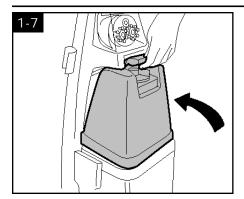
Replace clean solution tank (upper tank) by positioning bottom first. Press on tank handle to snap top of tank into place.
