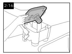
To remove tank lid, lower handle completely toward back of tank and lift off lid
