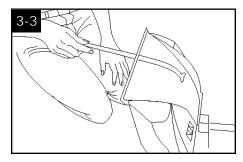
A nozzle clean-out tool, available at additional cost if not included with your cleaner, can be used for removing debris or if a non-carpeted floor is not available.
