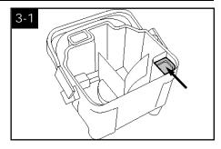
**d.** Remove lint from filter screen located inside recovery tank.
