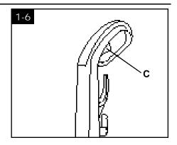
When handle sections are completely together, squeeze trigger (C) on upper handle.
