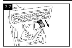
e. Remove lint from filter screen located on bottom of cleaner as follows. Note: When brushes seem to be rotating slowly, disconnect deep cleaner from electical outlet and check and clean this screen.
