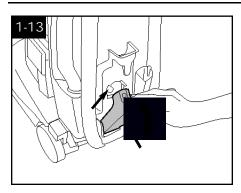
Position stair/upholstery nozzle in holder at base of cleaner and snap it into place as shown at arrow.
