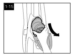
To remove powered hand tool, pull it down and outward.
