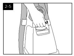
The deep cleaner may also be lifted by placing a hand under the upper clean solution tank handle as shown.
