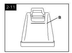
Pour detergent into tank. Fill tank to fill line (B) (1 gallon) with hot tap water.
