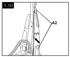
Press cord into cord clip on back of handle. Pull cord tight and wrap cord around hooks (A2).
