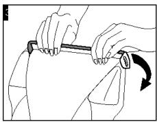
3. Push attachment against nozzle while rotating attachment downward until both ends snap into place.
