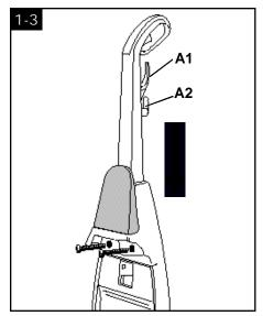
With hose hook (A1) and cord hook (A2) to back of deep cleaner, push upper handle down onto lower handle. Push **bolts** into holes on **front of handle. If bolts will not go through hole easily handle is not pushed completely down.**
