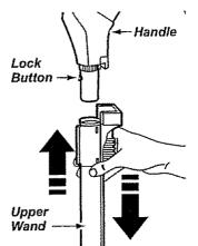
NOTE: If the Power-Mate® is attached, turn cleaner off before removing handle from wands.
