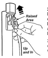
2. Connect Power-Mate<sup>®</sup> plug and cord as shown. **DO NOT force.** Raised area of plug must be toward hand.
