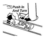
**2.** Push in and turn bulb counterclock-wise, then pull out to remove.
