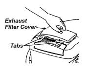
4. Replace the exhaust filter cover by engaging the two tabs on the rear and pushing down in front until it snaps closed.
