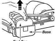
End Cap 7. Check and clean end cap areas. See AGITATOR ASSEMBLY for picture of complete agitator assembly.
