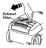
down until it snaps into place. Place the new filter into the motor cover with the **grey** edge down.
