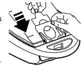
securely into the bag cavity so that none of it is able to be pinched by the hood.
