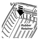
2. Replace the filter, rough side out, facing the dust bag, by sliding it back into place under the ribs in the bag cavity. Tuck filter in so that it fits completely under the rubber
