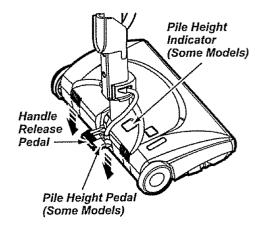
**3.** Lower wand from upright position by pressing on the handle release pedal.
