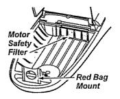
6. Check and replace, if necessary, the motor safety filter.
