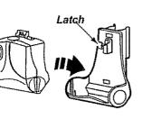
2. Rotate the Power-Mate Jr.<sup>®</sup> back until it snaps into place.
