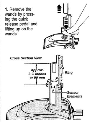
2. As indicated by the illustration, the two dirt sensor elements are located on the inside of the swivel, approximately 3½ inches/90 mm down, (note the arrows). Each element should be cleaned periodically. To reach the sensor elements, use a small brush such as a bottle brush. Brush each sensor element several times to remove dust and dirt.
