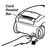
1. Pull cord out of canister to desired length. The cord will not rewind until the cord rewind bar is pushed.
