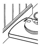
Active brush edge cleaners are on both sides of the Power-Mate<sup>®</sup>, Guide either side of the Power-Mate® along baseboards or next to furniture to help remove dirt trapped at carpet edges.
