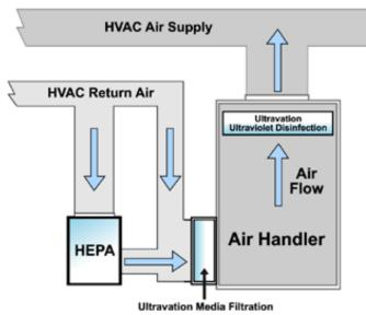
The Ultravation Photronic HEPA Air Cleaner has been designed for use in conjunction with virtually any HVAC system.
