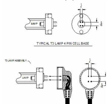
TYPICAL T3 LAMP 4 PIN CONNECTOR BASE
