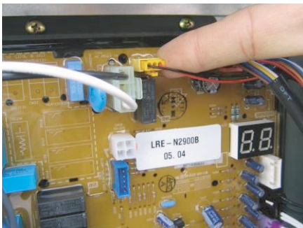
Position of cooling fan drive connector in main PCB
