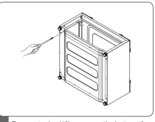
8 Remove twelve (12) screws on the bottom of the pedestal.
