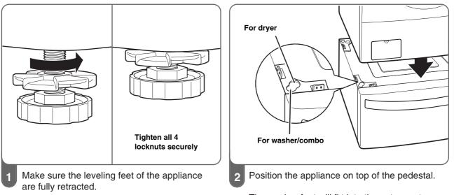
Once the leveling feet of the **washer** are fully retracted, tighten all locknuts securely.
