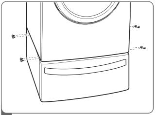
4 Make sure the holes on the pedestal align with the holes in the retainers, then install 2 screws at each corner to securely attach the appliance to the pedestal.
