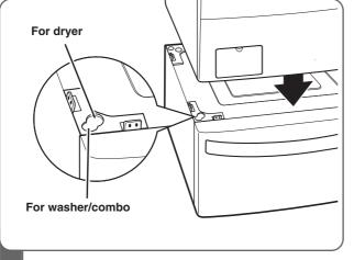
3 Place the dryer on the pedestal. Make sure the front and back feet are in the correct positions. The dryer feet will fi t into the innermost positions as shown.
