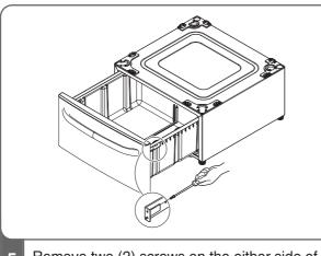
Remove two (2) screws on the either side of the drawer.
