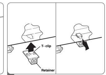
2 Insert the T-clip of the 4 retainers into the dryer base as shown. Press up on the back of the clip and pull outward to lock into place.
