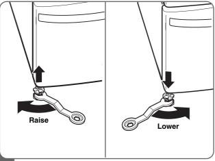
Loosen the locknuts on all 4 leveling feet of the **pedestal** until you can turn them with the wrench. Turn clockwise to raise or counterclockwise to lower until the pedestal is level and all 4 feet are solidly against the floor.
