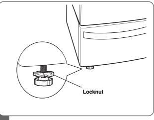
Securely tighten all locknuts by hand.
