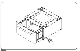
2 Open the drawer, and then remove the four (4) screws (two on each side) on both side of drawer.
