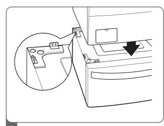
Make sure the back feet are in the correct positions.
