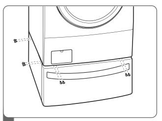
4 Make sure the holes on the pedestal align with the holes in the appliance, then install 4 screws at each corner to securely attach the appliance to the pedestal.
