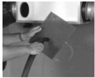
figure 17.2 Vacuum the Filters
