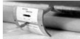
figure 13.4 Inserting Air flow grid in duct
