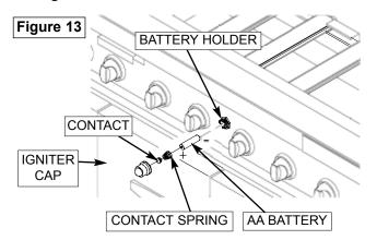
Place the Spring over the AA battery, then place the Contact on top of the Spring. Screw Igniter Cap(s) back onto the grill Control Panel.
