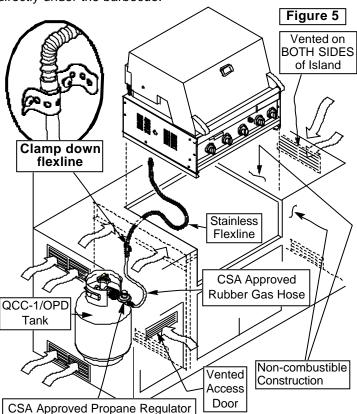
**NOTE:** Upper & lower ground-level vents (20 sq. in. minimum each) **MUST BE PROVIDED** for combustion air on both sides of built-in construction. Please ask a Barbeques Galore associate for full details.
