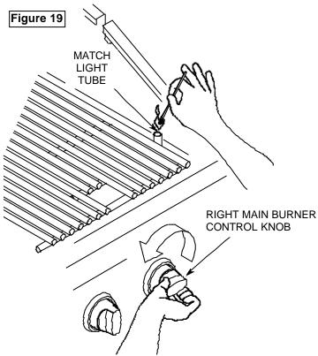
Occasionally observe the burner flame for correct operation. Once the right main burner is alight, the adjacent burner can be turned on and it will cross light off the operating burner. Repeat for each burner in turn. **Figure 19**
