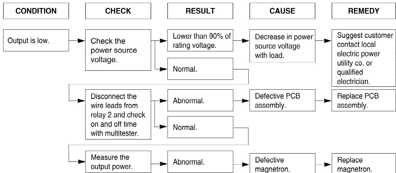
**NOTE :** Simple test of power output-conducted by heating one liter water for one min. if available.
