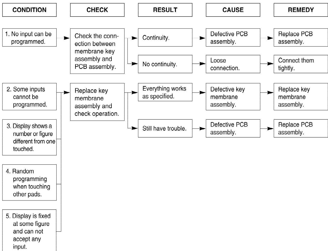
**(TROUBLE 2) Oven does not operate at all and Display window does not display any figures and no input is accepted.**
