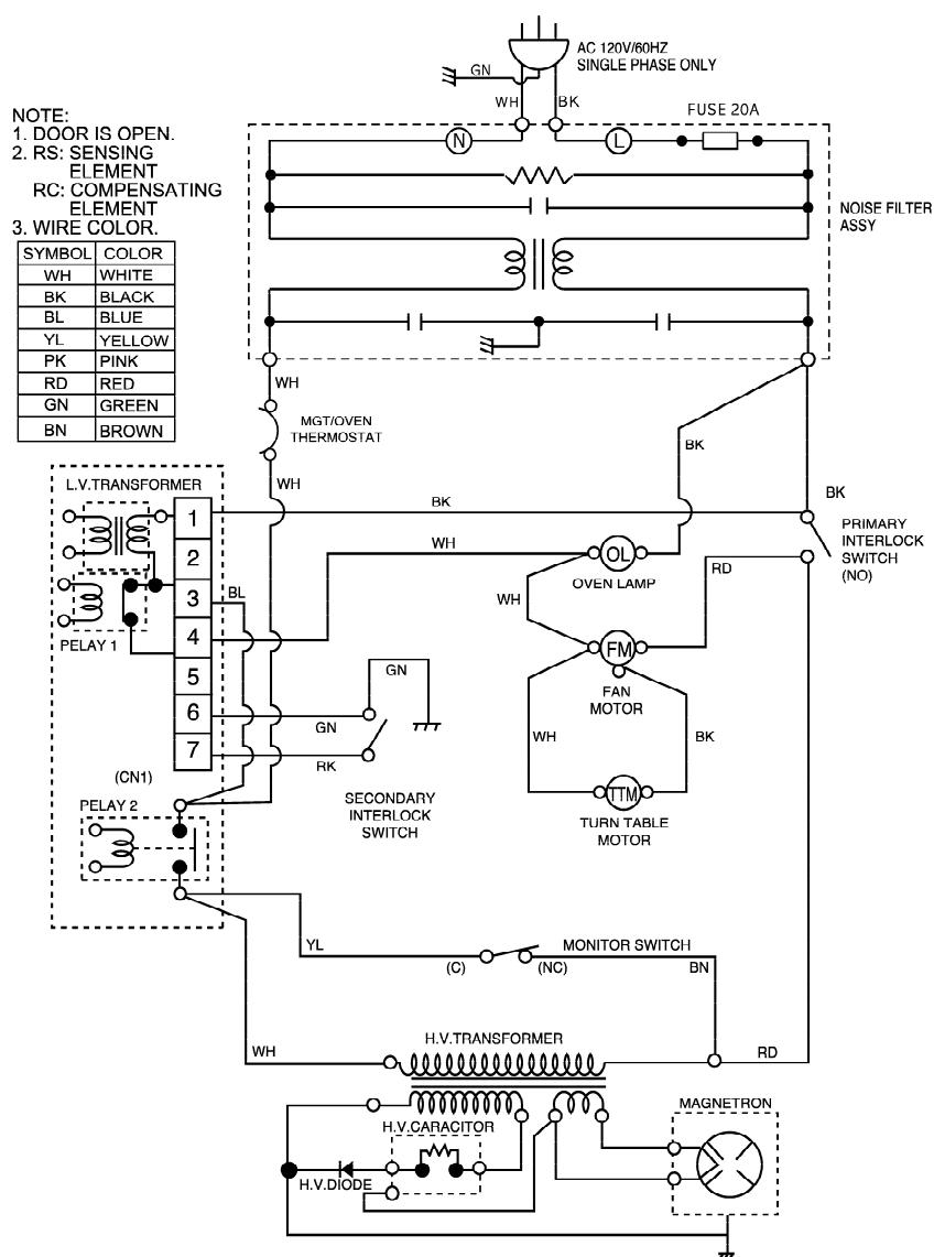
**IMPORTANT SAFETY NOTE:** THE SHADED AREAS ON THIS SCHEMATIC DIAGRAM INCORPORATE SPECIAL FEATURES IMPORTANT FOR PROTECTION FROM MICROWAVE RADIATION, FIRE, ELECTRICAL SHOCK, AND HAZARDS. WHEN SERVICING IT IS ESSENTIAL THAT ONLY MANUFACTURER'S SPECIFIED PARTS BE USED FOR THE CRITICAL COMPONENTS IN THE SHADDED AREAS OF THE SCHEMATIC DIAGRAM.
