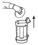
Remove foam filter from dirt container.
