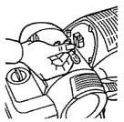
5. Pull bulb out of socket. Do NOT twist. Gently push replacement bulb into socket to replace.
