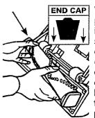
With new belt in place, pull and slide brushroll into nozzle making sure that the brushroll end caps are in the correct orientation (see diagram for end cap orientation). Rotate brushroll manually to make sure belt is properly aligned.
