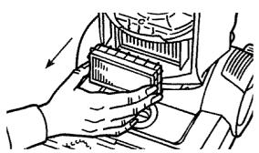
Return exhaust filter to cleaner. Replace exhaust filter cover by inserting the tab on the cover into the slot on the cleaner. Pivot toward cleaner until cover snaps into place.
