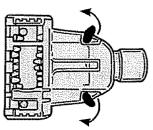
To reassemble, align tabs on the lower housing with the slots on the cover and pivot cover back into position on top of lower housing. Rotate locking tabs inward into locking position.
