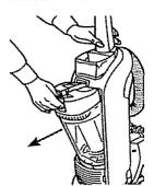
Press dirt container release button and remove dirt container from cleaner.
