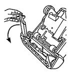
Rotate/pivot the nozzle guard and pull off
