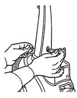
2. Push handle plug onto the front of cleaner. Insert the one (1) screw into the back of the handle and tighten, making sure the handle plug is secure.
