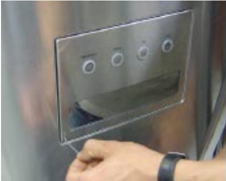
1) With the unit unplugged from the power source, you can manually open the dispenser cover using a small flat blade screwdriver. The cover will remain opened during the repair.
