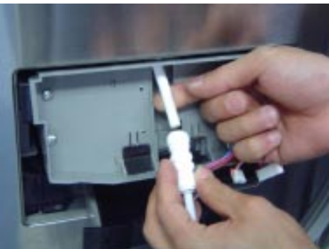
5) Separate tube (5/16") from connector (clip have to be removed first)
