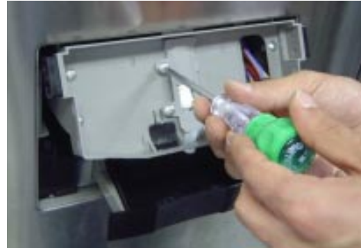
4) Unscrew 2 points and then remove connector-cover
