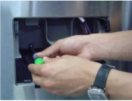
7) Unscrew 2 points to separate tray-cover
